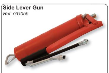
For 400g Cartridges or 500g Bulk fill Metered Output, Permanent Spring Load Design, Filler Nipple, Air Release Valve, Plastic Hand Grip. 1/8"BSP Thread C/w Rigid & Flexible Tube & 4 Jaw Hydraulic Connector
